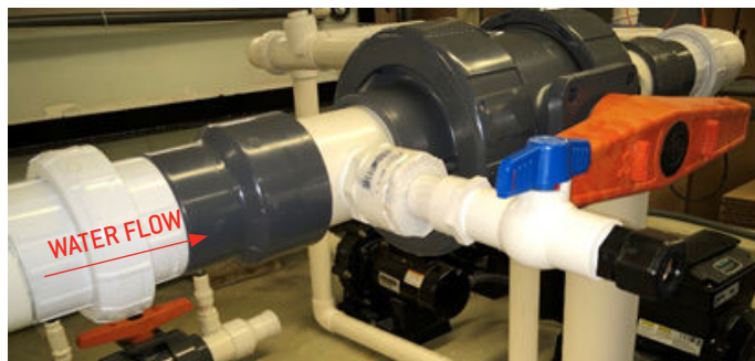
Inlet water pitot tube - notch facing downstream
