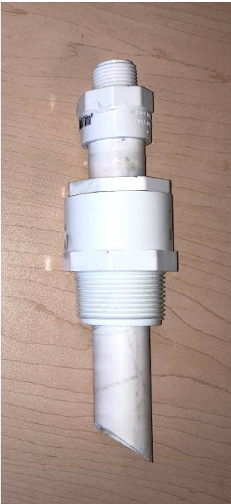
Pitot Tube – 2 5/8” For 3” pool piping
