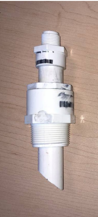
Pitot Tube – 1 7/8” For 2 ½” pool piping
